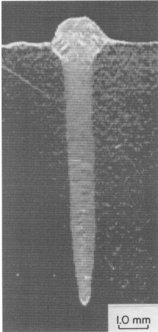
Fig. 2 Transverse cross section (i.e., yz -plane) of weld showing penetration depth and transverse extent of solidified melt pool. For this system, V_B = 3 cm/s, and the power into workpiece is \sim 3 kW. The depth of penetration is 7.75 mm (0.305 in.)
